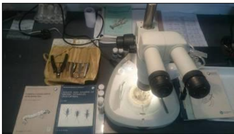
Plate 1.1 – Nikon SMZ 1000 microscope and FBA keys used for macro-invertebrate identification
